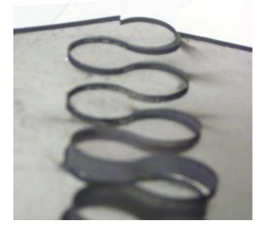
Figure 2. Balance between fitting tolerances and the constraints of assembly tolerances. The first nodes lock into place but prevent the following nodes to reach their position due to a fitting tolerance that is too tight.
