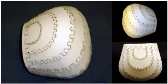
Figure 1. Example of puzzle joint surface
