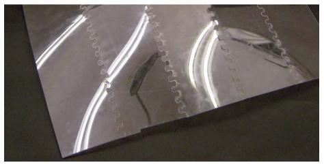
Figure 11. Reflection lines show the distortion of the developable strips into partial double curvature due to the joints bridging the ridge between the strips.
