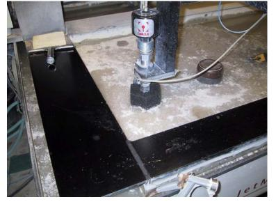
Figure 10. Cutting of the polycarbonate pieces in an OMAX<sup>TM</sup> water jet cutter
