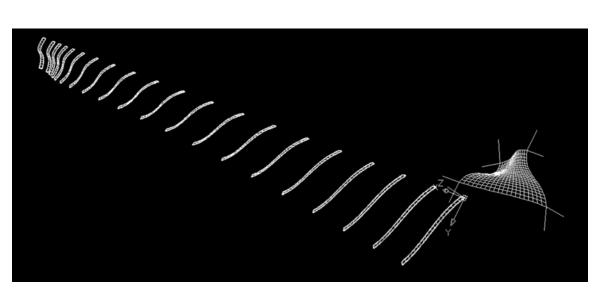
Figure 7. After running the fabrication script over the surface 20 strips are flattened out
