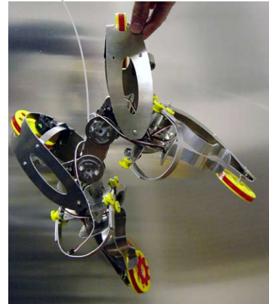
Eight DOF redesign physical mockup incorporating the changes. Change of fabrication triggers further design changes.
