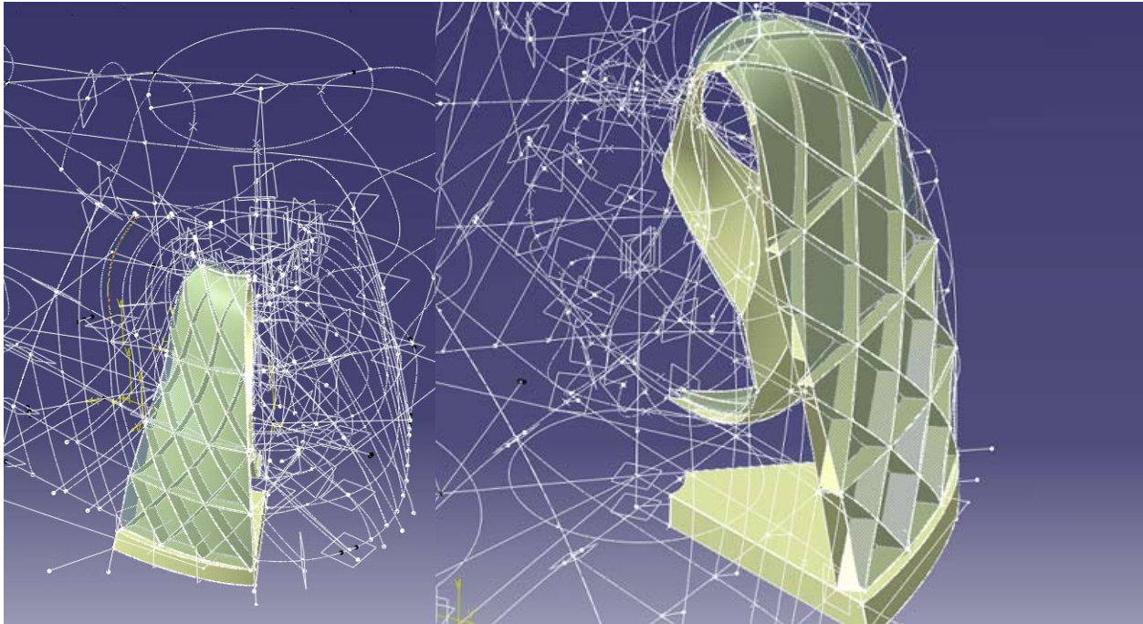
The hierarchical control grid for the pavilion. It allows the high level edit of the overall layout of the pavilion through the positioning of the floor plan. Image: Axel Kilian
