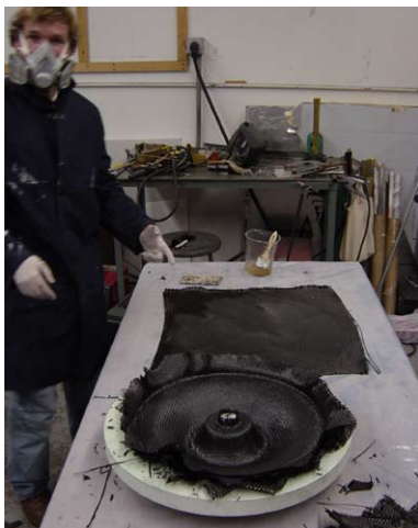
Fabrication of the full scale design in carbon fiber based on molds in mdf and soft foam plugs. All molds and plugs were CNC milled.
